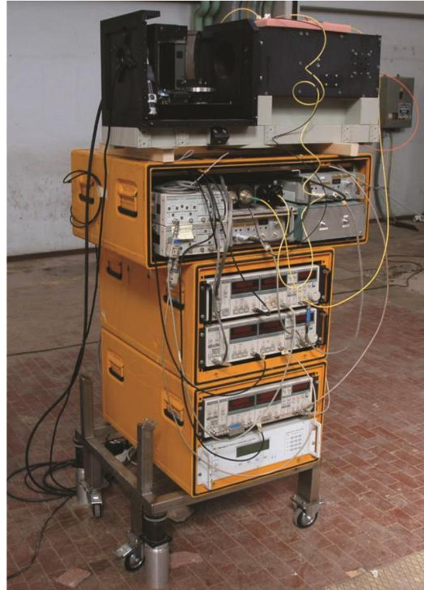
Most of the actual limitations derive by the choice of commercial instruments designed for general purpose laboratory/bench usage *but not for field deployment*.
