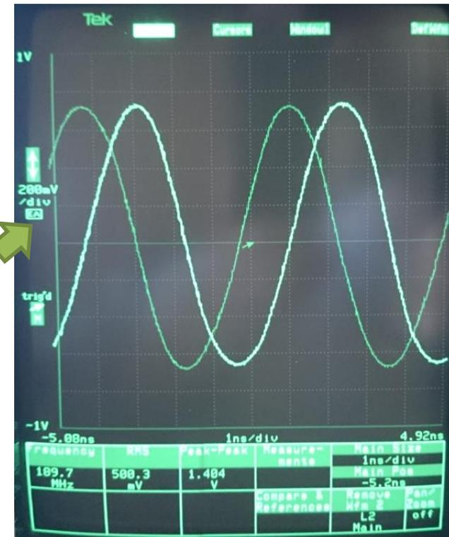
(center)  $R_E$  (in phase) channel; (right)  $I_M$  (in quadrature) channel. The amplitudes are (in terms of RMS voltage) practically equals (500 mV = +7dBm). The two waveforms are exactly in quadrature. [EA] (Extended Accuracy) means 10 bit accuracy.
